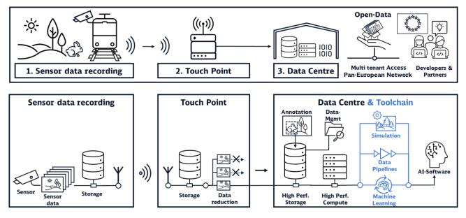
Figure 6. Flow of data from sensor recordings to trained AI models.
